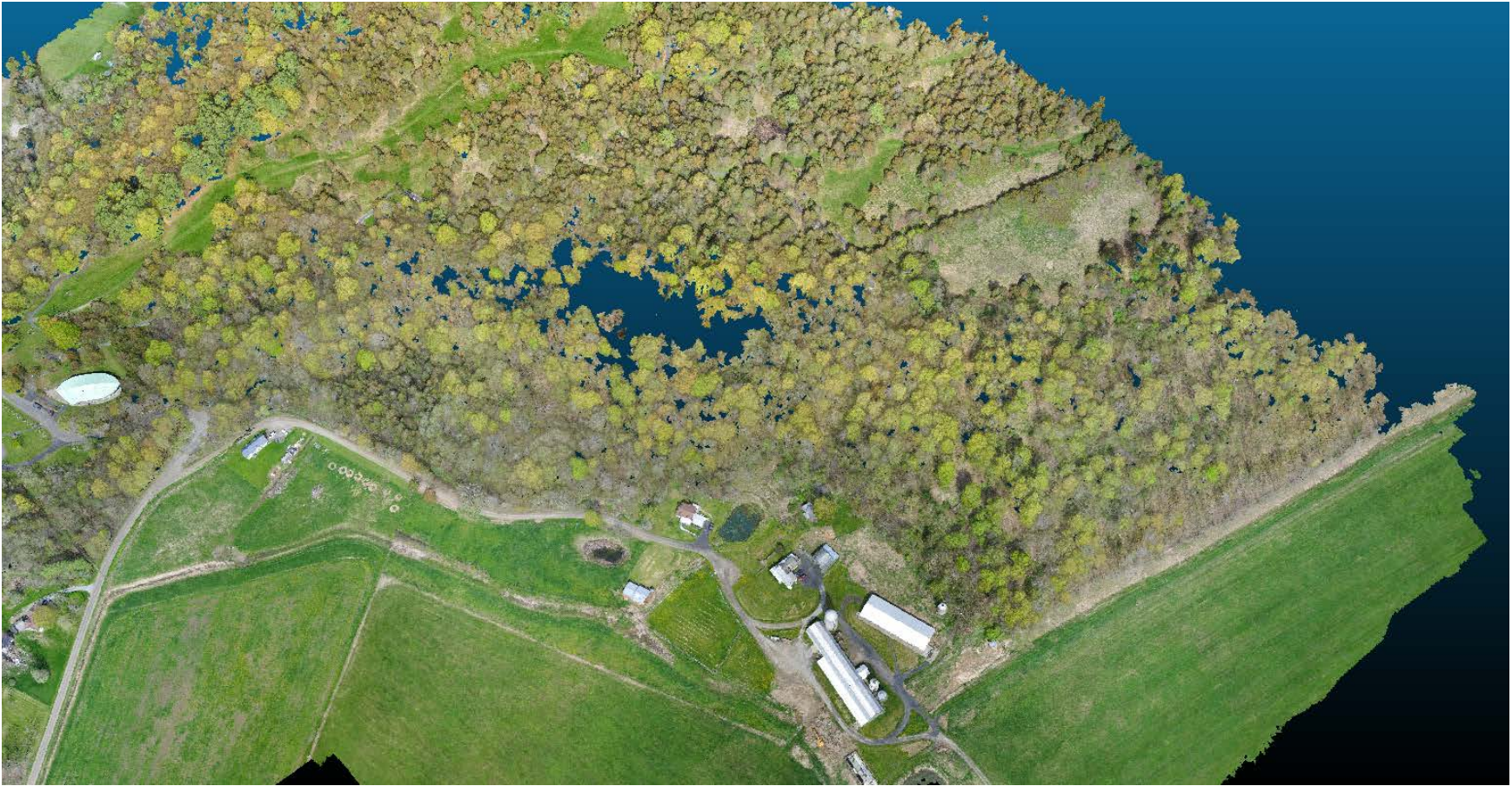
Figure 7. Photogrammetrically derived “point cloud” generated from imagery taken by UVM SAL’s unmanned aircraft system.
