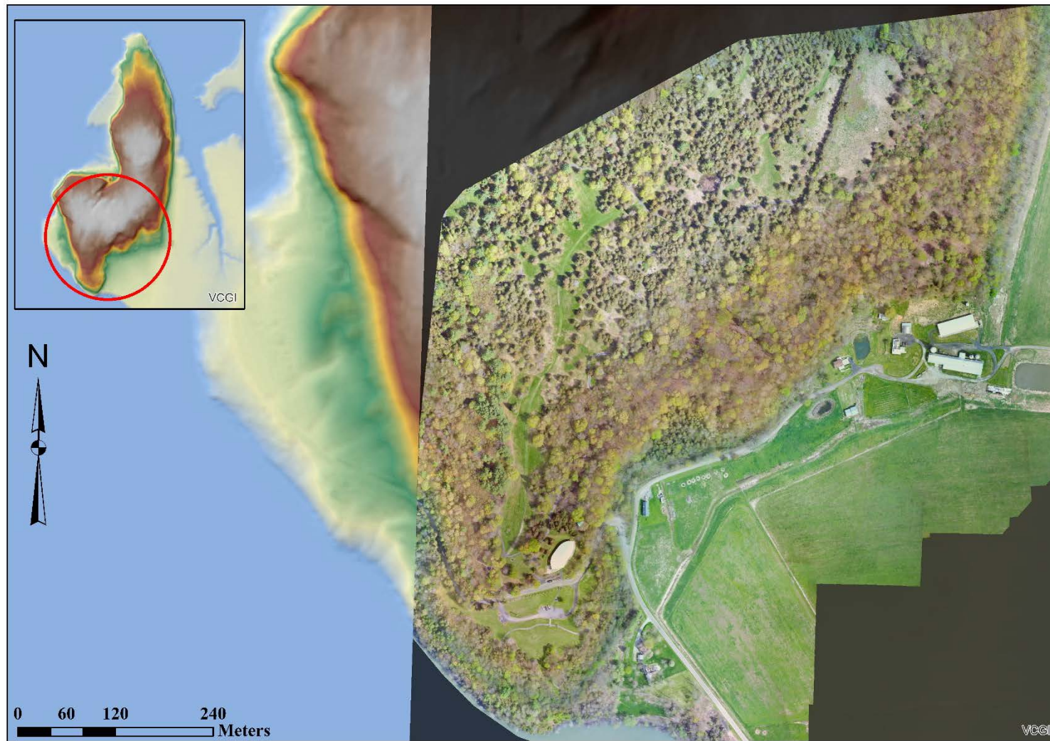
Figure 7. High-resolution orthoimage of the southern portion of Mount Independence constructed from UAS photographs.
