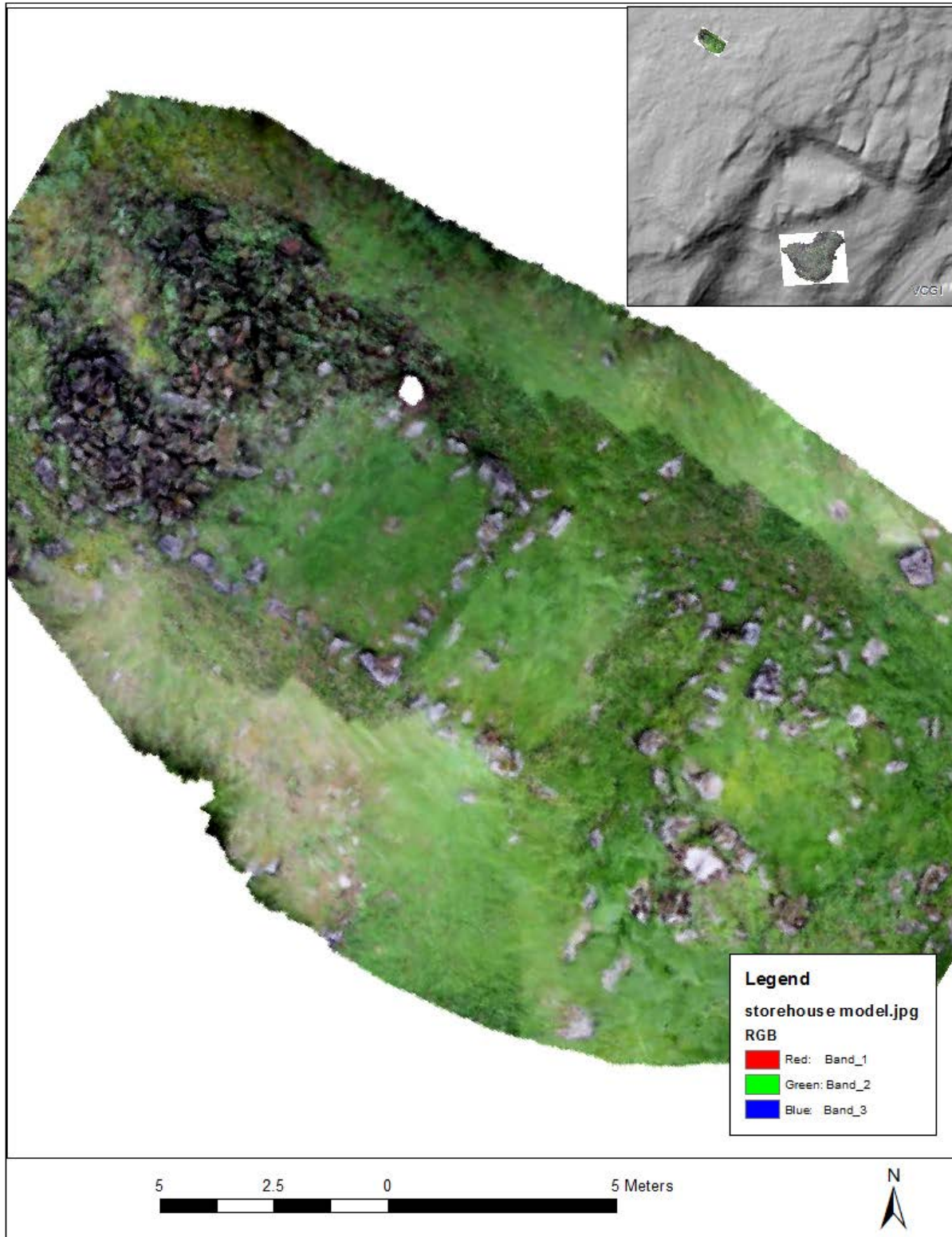
Figure 25. Plan view of photogrammetric textured mesh model of Mount Independence storehouse rendered from hand-held digital SLR imagery. Inset shows storehouse on LiDAR imagery in relation to 2 nd Battery.
