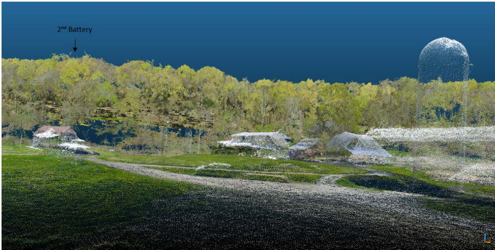
Figure 11. Three-dimensional view of point cloud generated from UAS flight data. The location of the second battery is indicated. Image reproduced from UVM CAP's technical report. See Appendix A.
