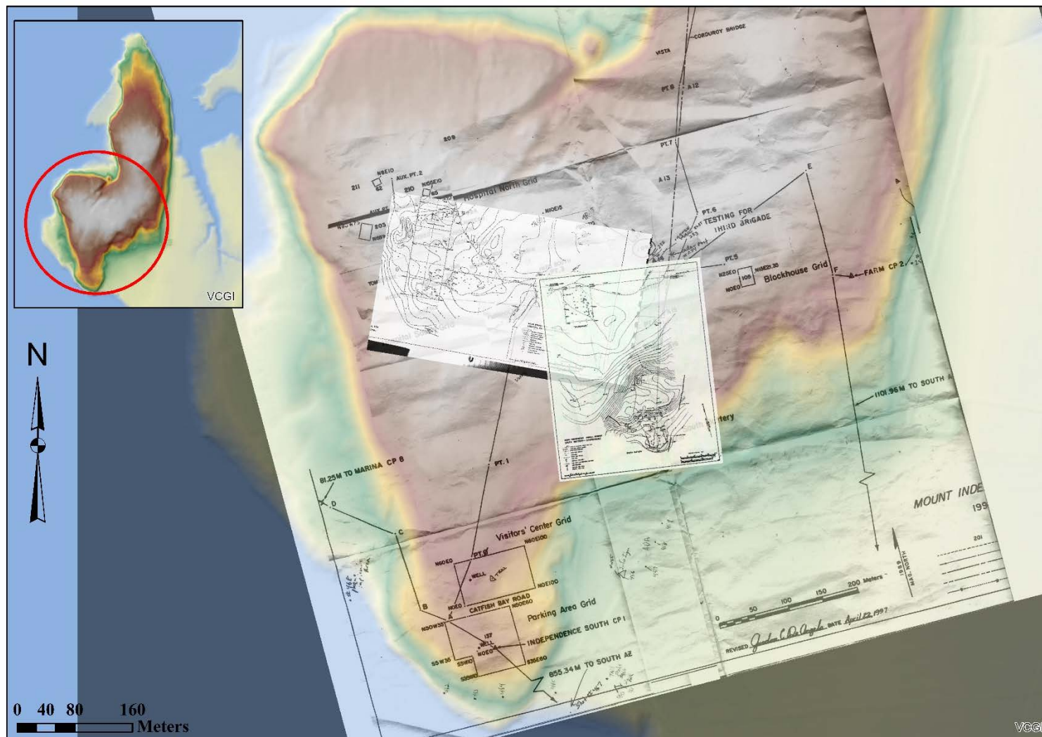
Figure 15. Composite georeferenced maps overlying modern LiDAR imagery of the Mount.
